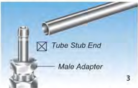
To eliminate the problem, use a male adapter into the female port.
