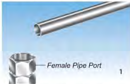
In the direction shown the female port is required to connect with tubing.
